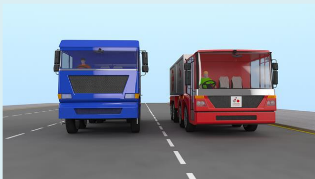
Figure 12; comparison between a traditional construction HGV and its possible redesign with lower, better placed cab 23
